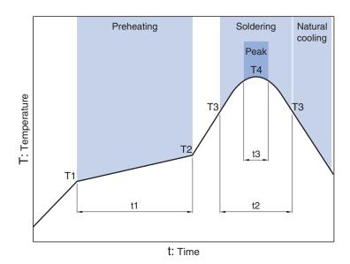
Soldering Preheating Peak Temp. Time Time Temp. Time Temp. T2 **T3** T4 t3 150°C 180°C 120s 230°C 30s 260°C 10s max.
